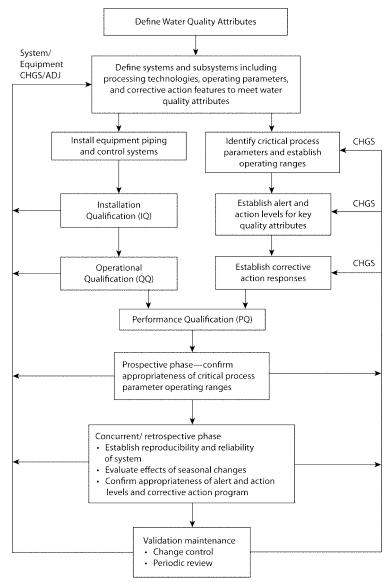
Figure 3. Water system validation life cycle.
